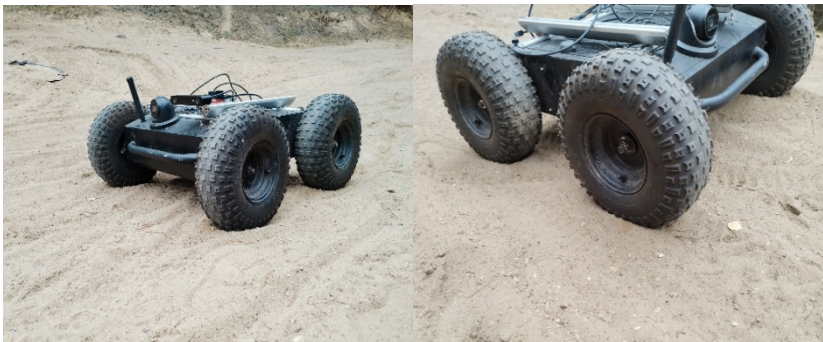
Fig. 10 Field test of the wheeled mobile robot on sandy terrain
