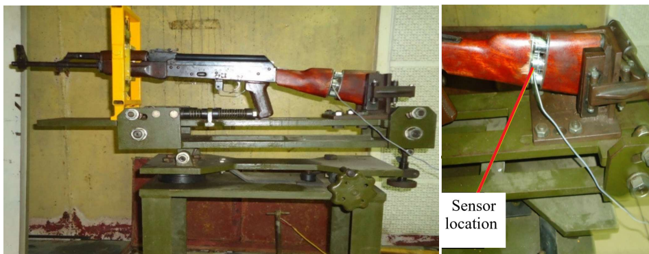
Fig. 5 Experimental measurement of gun recoil force
