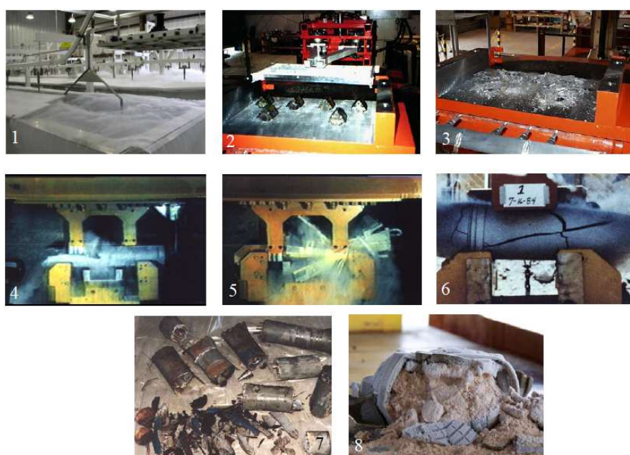
Fig. 14 Stages of cryogenic demilitarization [37]
