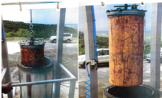
Fig. 11 Extraction of explosive filler from a munition [31]
