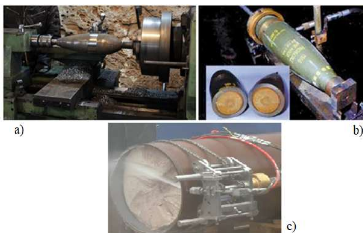
Fig. 10 Mechanical disassembly: (a) lathe operation for case removal; (b, c) water-abrasive cutting [29, 30]
