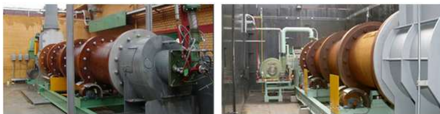
Fig. 3 Rotating incinerator for explosive waste (EWI – APE 1236) [15]
