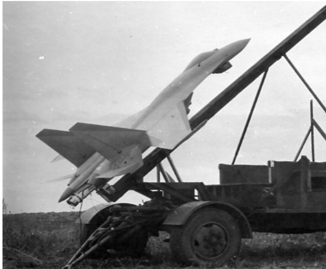
Fig. 2 FDSM SLMT-10S-BP of the Su-27 aircraft on the ground launch rig
