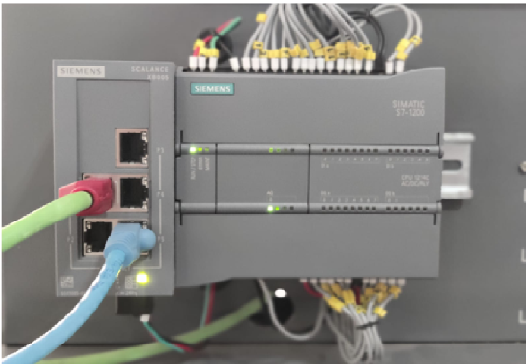
Fig. 2 Siemens SIMATIC S7-1200 PLC
