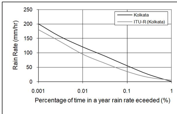
Fig. 5 Rain rate statistics for Kolkata: obtained experimentally and from the ITU-R model
