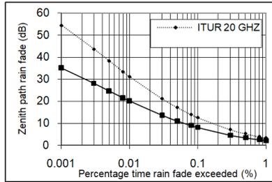
Fig. 12 Zenith path rain fade using RBSM & ITU-R model at 20 GHz
