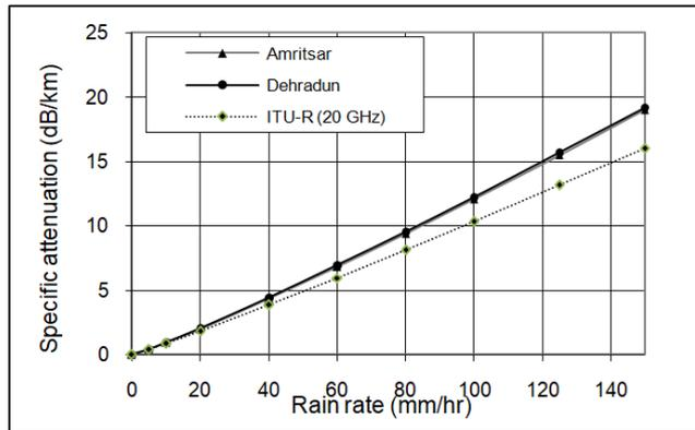
Fig. 6 Comparison of measured specific attenuation with ITU-R model at 20 GHz
