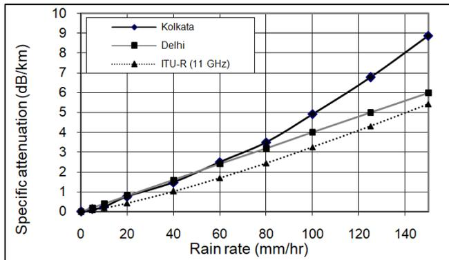
Fig. 7 Comparison of measured specific attenuation with ITU-R model at 11 GHz
