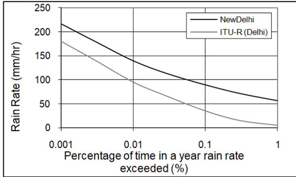
Fig. 4 Rain rate statistics for New Delhi: obtained experimentally and from ITU-R
