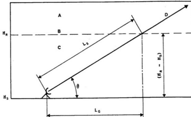
Fig. 1 Schematic of earth space slant-path
