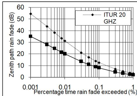
Fig. 2 Rain rate statistics for Amritsar: obtained experimentally and from ITU-R model
