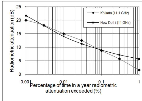
Fig. 9 Cumulative distribution of radiometric attenuation at 11 GHz
