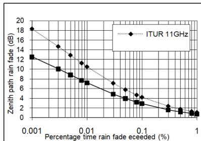
Fig.13 Zenith path rain fade using RBSM & ITU-R model at 11 GHz
