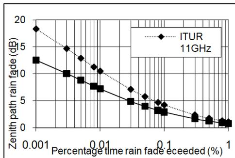
Fig. 3 Rain rate statistics for Dehradun: obtained experimentally and from the ITU-R model
