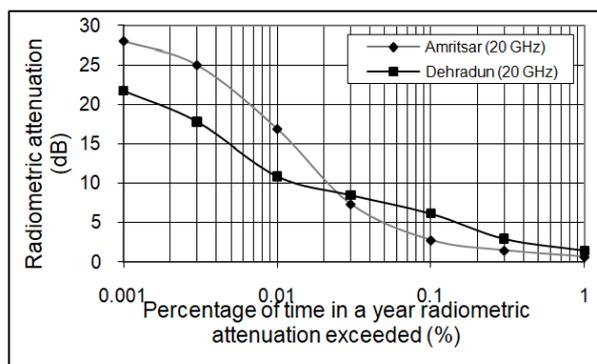
Fig. 8 Cumulative distribution of radiometric attenuation at 20 GHz
