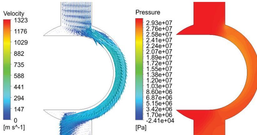
Fig. 15 Velocity vectors and pressure distribution in the vent of regulator for  $p_b > p_c$
