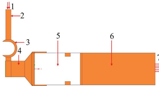
Fig. 5 CFD model of the gas-operated mechanism of UK-59 machine gun: 1 – inlet; 2 – gas port; 3 – gas vent of regulator; 4 – gas cylinder; 5 – piston; 6 – flow space behind the piston; 7 – outlet
