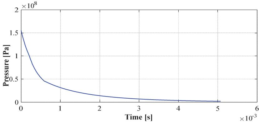
Fig. 6 Pressure of inlet propellant gases
