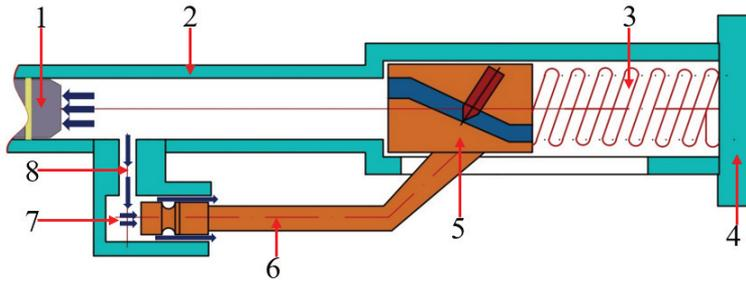
Fig. 1 Schema of the gas-operated automatic weapon drive: 1 – projectile; 2 – barrel walls; 3 – return spring; 4 – weapon casing; 5 – breech block carrier; 6 – piston; 7 – gas cylinder; 8 – gas port
