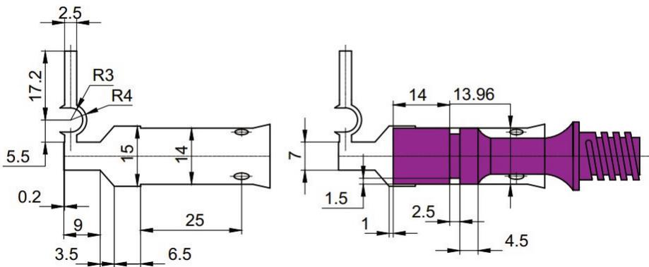
Fig. 4 Geometric dimensions for the UK-59 machine gun
