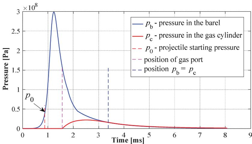
Fig. 2 Typical evolutions of gases pressure in the barrel and in the gas cylinder
