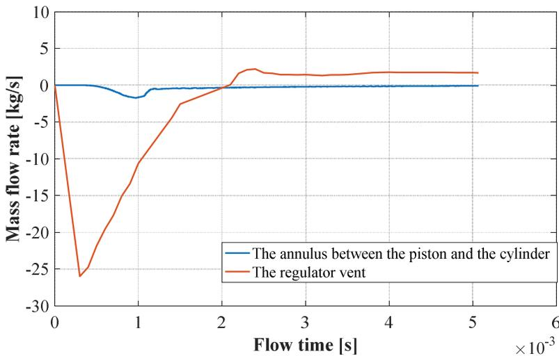
*Fig. 18 Mass flow rate of gases flowing through the regulator vent and through the annulus between piston and cylinder versus time*
