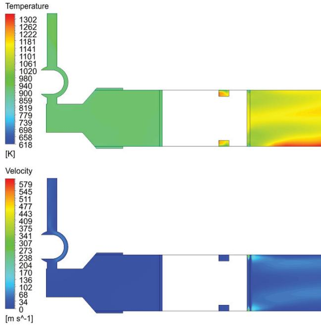
*Fig. 13 Temperature and velocity distribution in gas-operated mechanism for time  $t = 3$  ms and piston displacement  $x_p = 15.2$  mm*
