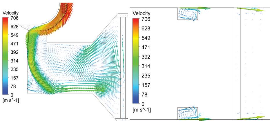
Fig. 17 Velocity vectors of the propellant gases flow in the cylinder and in the annulus between the piston and the cylinder for  $p_b > p_c$
