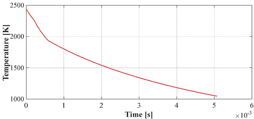
Fig. 7 Temperature of inlet propellant gases
