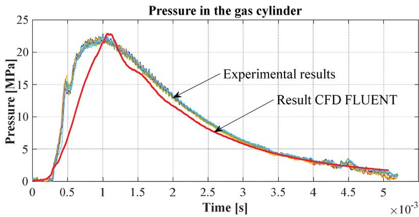
Fig. 9 Comparison of the evolution of the gas cylinder pressure by CFD simulation and experiment for UK-59 gas-operated mechanism
