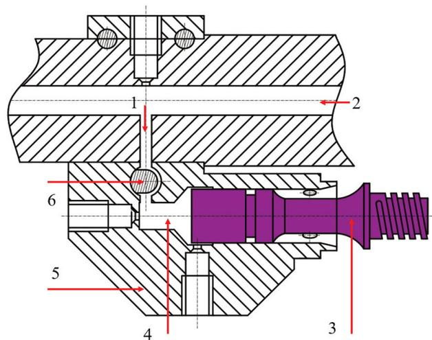
*Fig. 3 The gas-operated mechanism of UK-59 machine gun: 1 – gas port; 2 – barrel; 3 – piston; 4 – gas cylinder; 5 – gas block; 6 – regulator*
