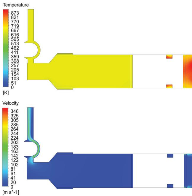
*Fig. 14 Temperature and velocity distribution in gas-operated mechanism for time  $t = 5.07$  ms and piston displacement  $x_p = 30.5$  mm*
