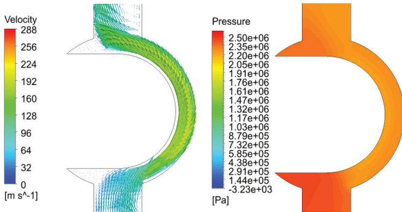
Fig. 16 Velocity vectors and pressure distribution in the vent of regulator for  $p_b < p_c$
