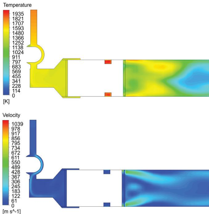
*Fig. 11 Temperature and velocity distribution in gas-operated mechanism for time  $t = 1$  ms and piston displacement  $x_p = 0.75$  mm*
