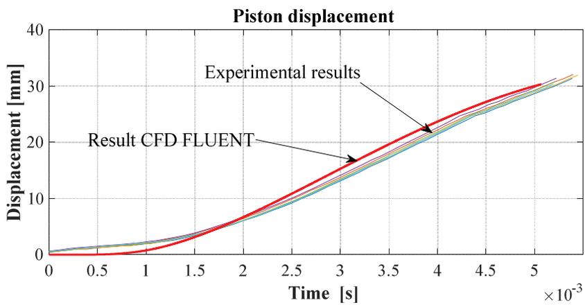
Fig. 10 Comparison of the piston displacement by CFD simulation and experiment for UK-59 gas-operated mechanism
