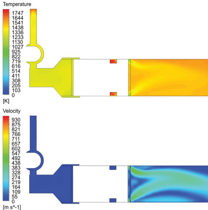
Fig. 12 Temperature and velocity distribution in gas-operated mechanism for time  $t = 1.5$  ms and piston displacement  $x_p = 3.07$  mm
