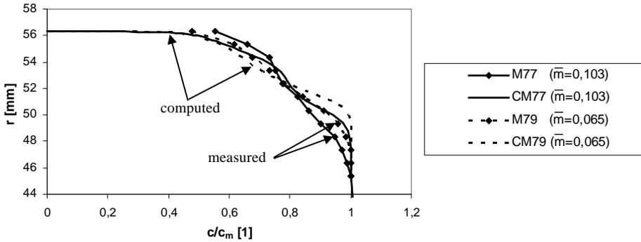
Fig. 16 Comparison of calculations and measurements for  $b_2 = 90^\circ$  [13]
