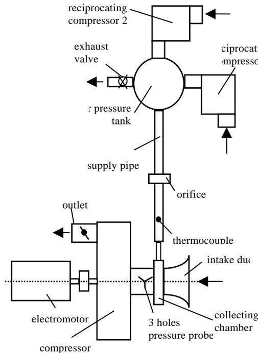
Fig. 3 Scheme of the test bench [9]
