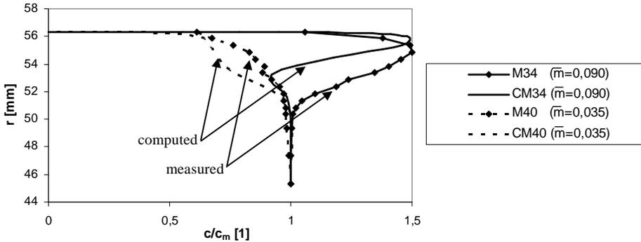
Fig. 15 Comparison of calculations and measurements for  $b_2 = 20^\circ$  [13]
