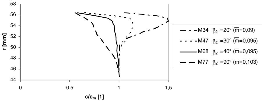
Fig. 9 Influence of angle  $b_2$  on velocity field for higher relative mass flow rate [9]
