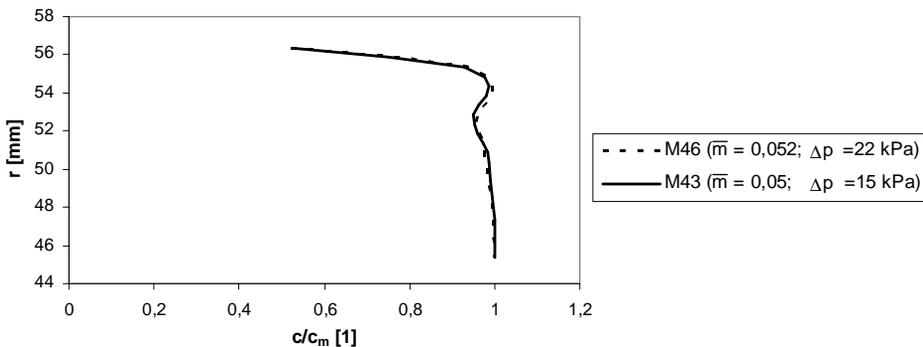
Fig. 8 Influence of pressure drop  $\Delta p$  on velocity field for angle  $b_2 = 20^\circ$  [9]
