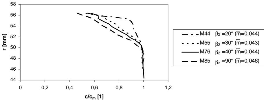
Fig.10 Influence of angle  $b_2$  on velocity field for lower relative mass flow rate [9]
