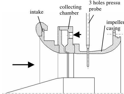
Fig. 4 Scheme of the intake system with collecting chamber [9]
