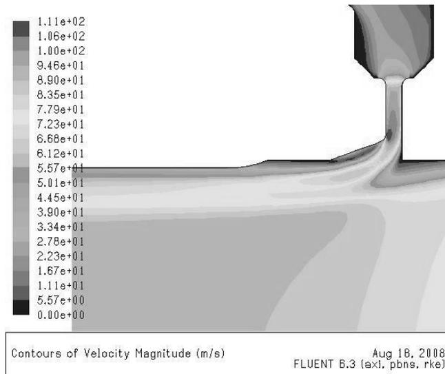
Fig. 14 Velocity field distributions with slot angles  $b_2 = 90^\circ$  (CM77) [13]
