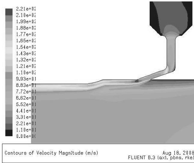
Fig. 13 Velocity field distributions with slot angles  $b_2 = 20^\circ$  (CM34) [13]
