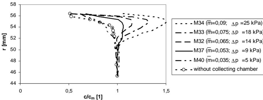
Fig. 7 Influence of relative mass flow rate on velocity field for angle  $b_2 = 20^\circ$  [9]
