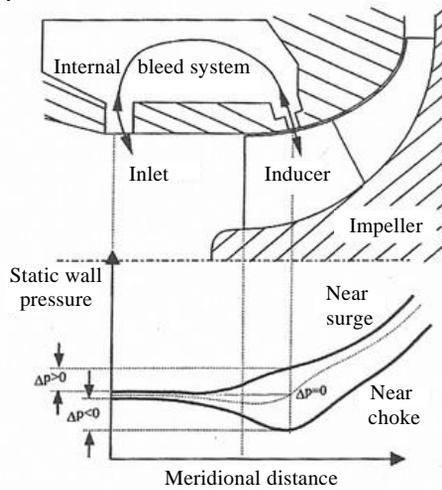
Fig. 1 Scheme of air flow in the bleed system [8]
