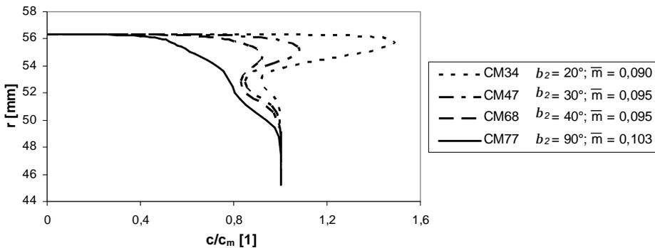
Fig. 12 Calculated velocity field distributions for different slot angles  $b_2$  [13]
