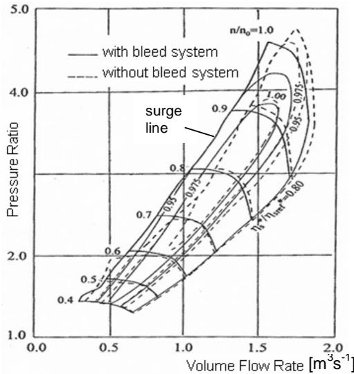
Fig. 2 Compressor characteristics with and without bleed system [8]
