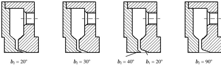
Fig. 5 Versions of collecting chamber with slot
