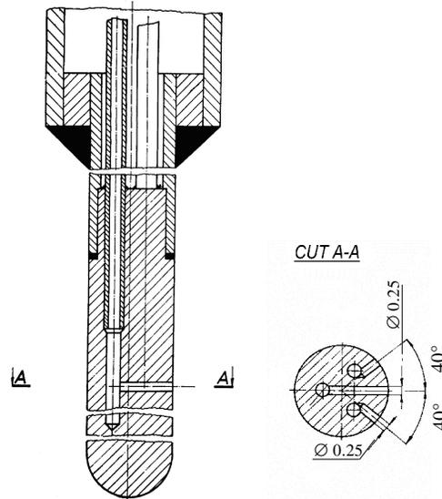
Fig. 6 Scheme of 3 holes pressure probe [9]
