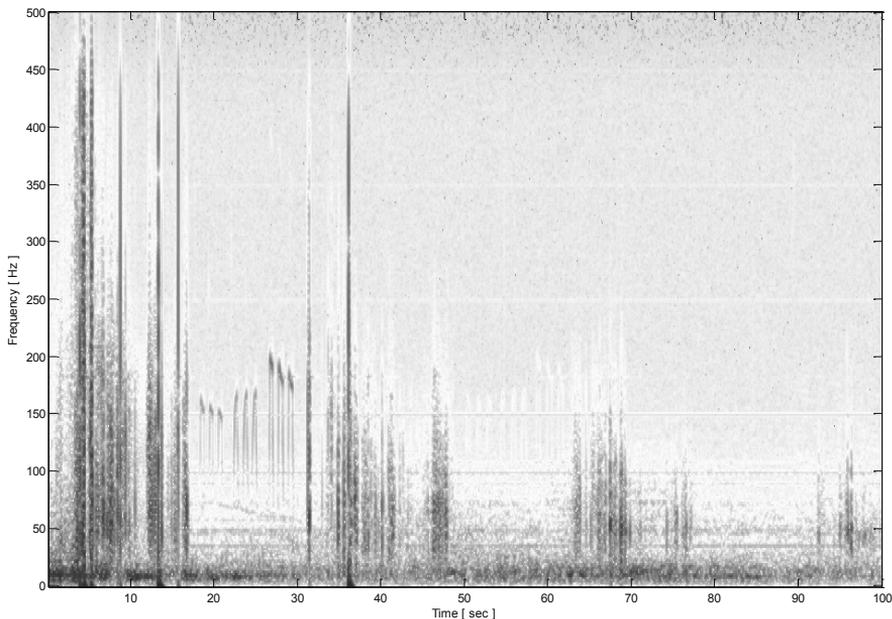
*Fig. 5 Spectrogram of seismic surface wave signals, vertical orientation*
