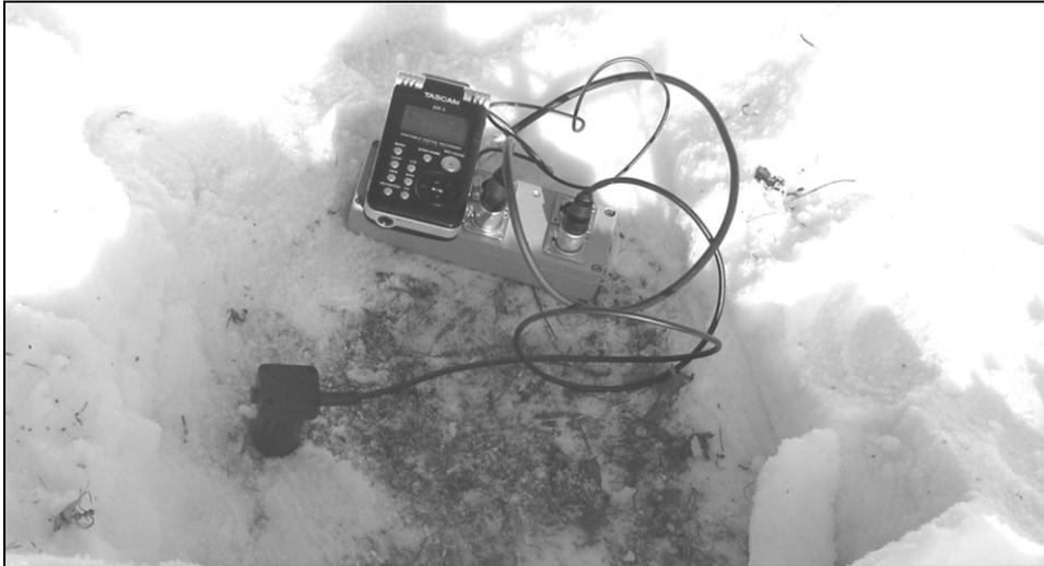
*Fig. 4 Photograph of measurement point (SM-6 geophone, amplifier, DR-1 recorder)*
