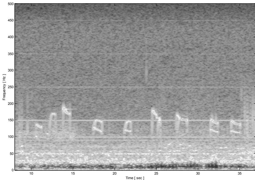
*Fig. 7 Spectrogram of seismic surface wave signals, horizontal orientation, and combination of vibration motors switched on*
