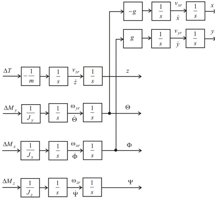
Fig. 3 Structure of linearized controlled plant
