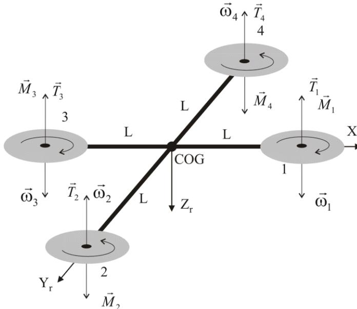
Fig. 1 Kinematic scheme of the quadrotor
