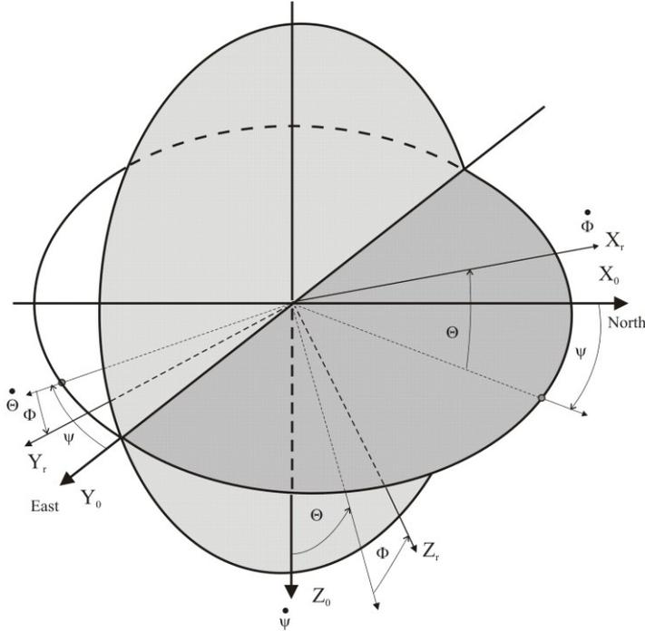
Fig. 2 Orientation of frames
