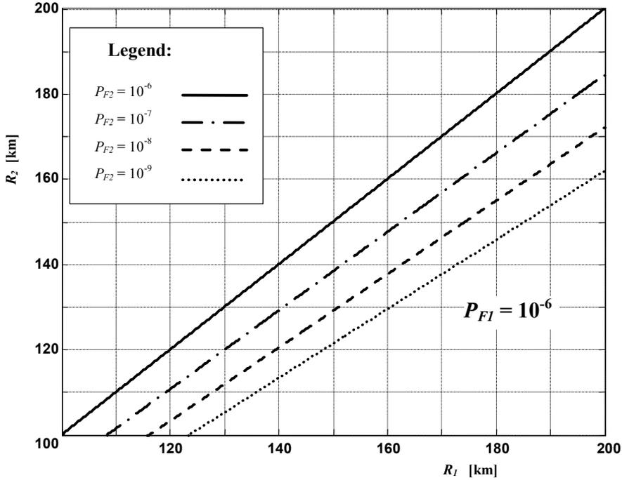
Fig. 3 Graph of dependency  $R_2 = f(R_1)$  on  $P_{F2}$  for  $P_{F1} = 10^{-6}$
