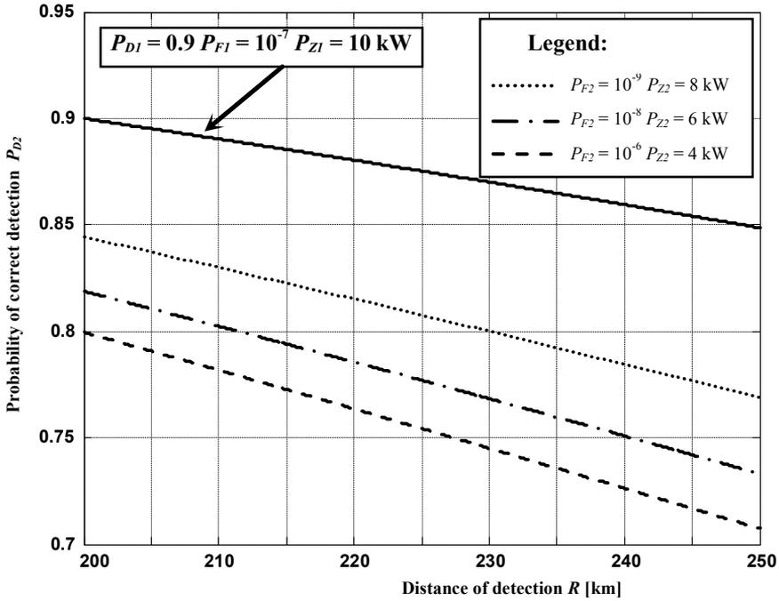
Fig. 5 An example of the simulation results for  $P_{D2}$  in the ELINT systems with the selected parameters  $P_Z$ ,  $P_D$  and  $P_F$
