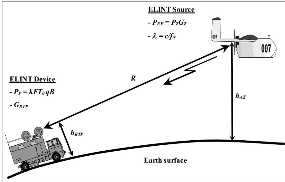
Fig. 1 ELINT system configuration
