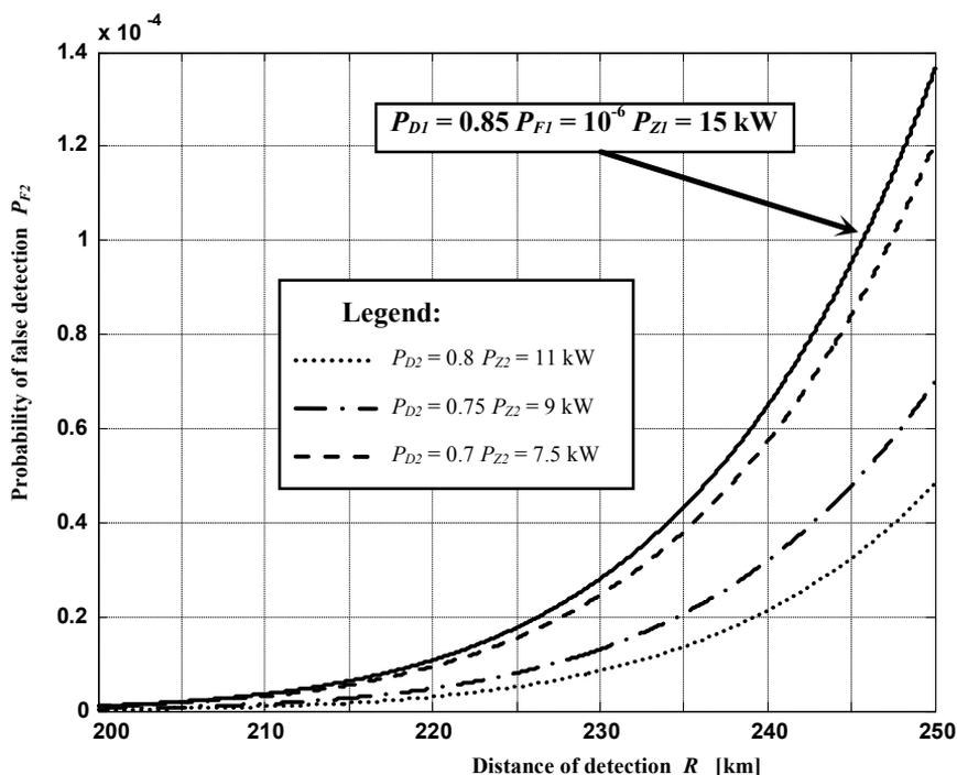
Fig. 6 An example of the simulation results for  $P_{F2}$  in the ELINT systems with the selected parameters  $P_Z$ ,  $P_D$  and  $P_F$
