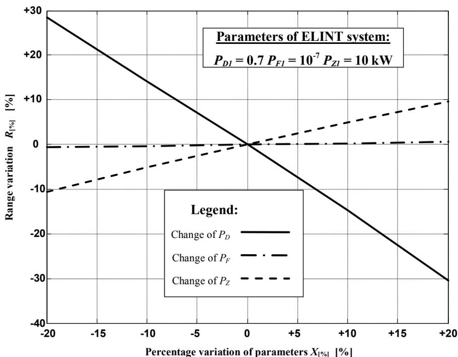
Fig. 7 The graphic dependency of range variation  $R_{[%]}$  of ELINT system on variation of parameters  $X_{[%]}$
