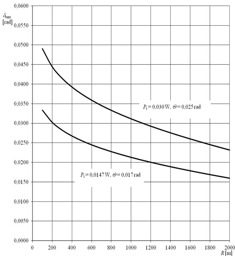
Fig. 4 Course of the limit angular beam deflection
