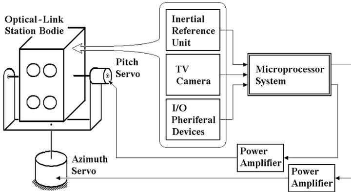
Fig. 7 Structure of the control system of the FSO station motion
