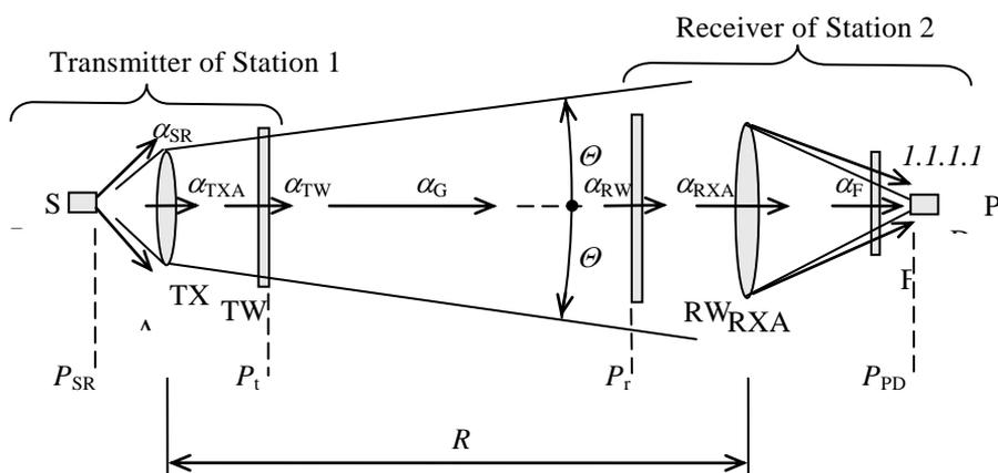
Fig. 1 Arrangement of one channel of the FSO link [1]
