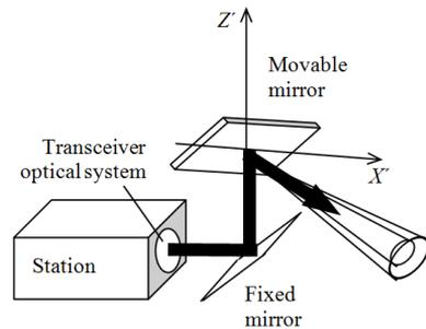
Fig. 6 Control of the optical axis of the FOS link by means of an assemblage of mirrors
