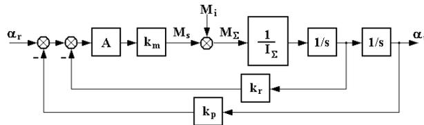
Fig. 8 The block diagram of the servomechanisms of the FSO stations
