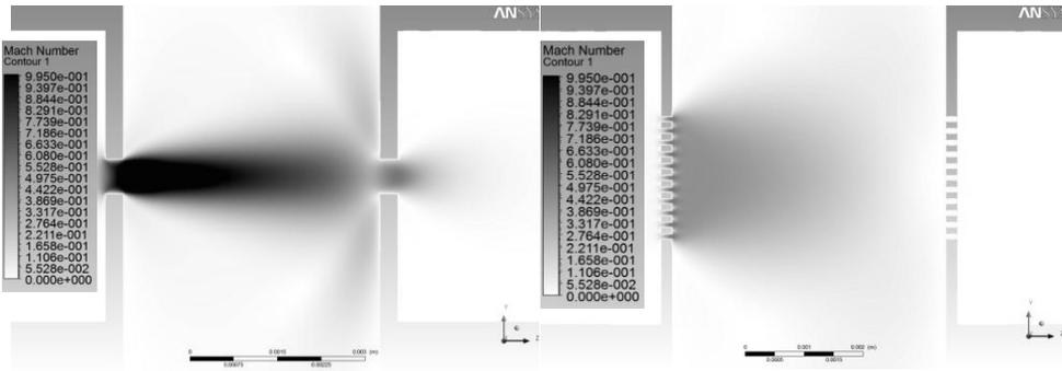
Fig. 7: Speed distribution characterized by Mach number for variant with one hole of 0.6 mm in diameter (left) and for variant with 127 holes of 0.1 mm in diameter (right).
