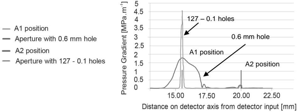
Fig. 6 Comparison of gas pressure gradient on detector axis.
