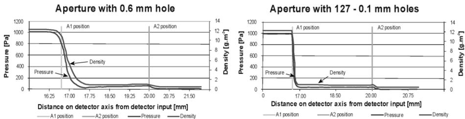
Fig.3 Gas pressure and gas density dependence along the detector axis
