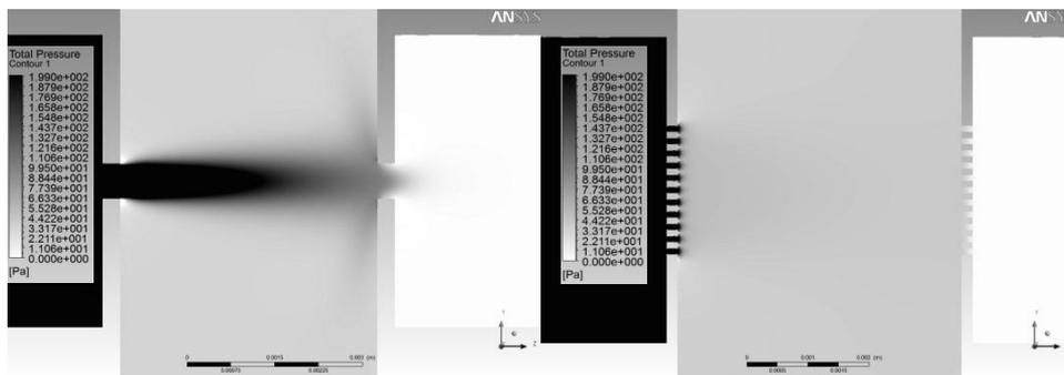
Fig. 8 Comparison of total pressure distribution for variant with one hole of 0.6 mm in diameter (left) and for variant with 127 holes of 0.1 mm in diameter
