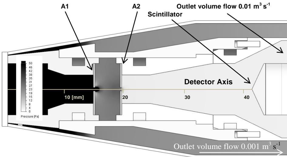
*Fig. 1 Distribution of gas pressure in SEs scintillation detector for ESEM*
