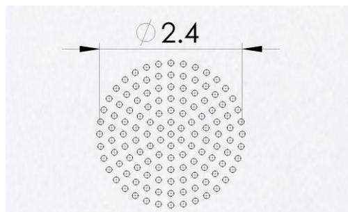
*Fig. 2 Positioning of holes with diameter of 0.1 mm round the centre of apertures A1 and A2.*
