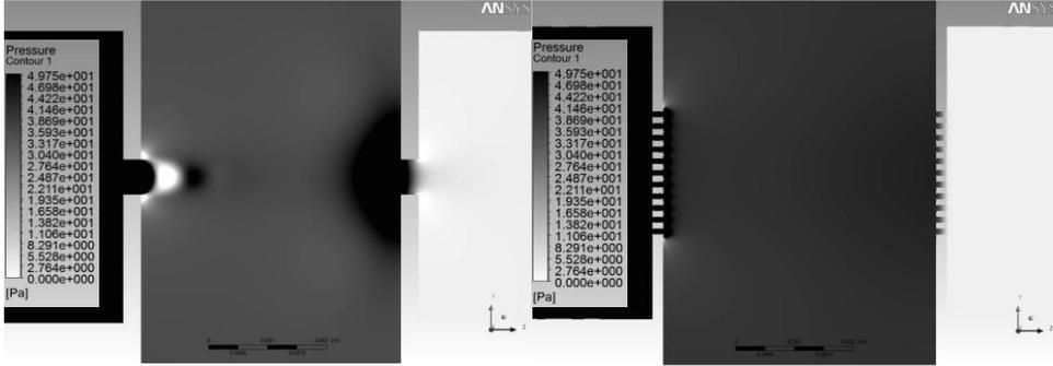
*Fig. 4 Magnitude and distribution of static gas pressure in the space between apertures A1 and A2 for variant with one hole of 0.6 mm in diameter (left) and for variant with 127 holes of 0.1 mm in diameter (right).*
