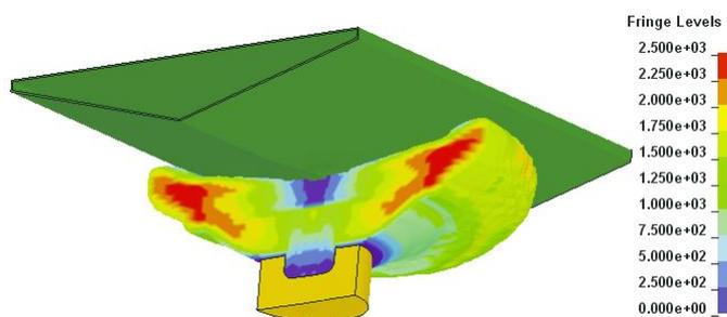
*Fig. 1 Ballistic load of structure (frame)*
