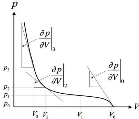
Fig. 2 Nonlinear compression curve of a solid elastic-plastic material allowing for dispersion driven shock waves (Reproduced with permission of Author [2])
