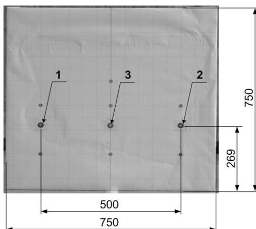
Fig. 1 Reference points and size (in millimetres) of the model of target
