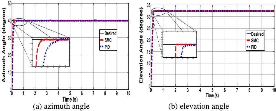
Fig. 13 Controllers performance using ideal actuator
