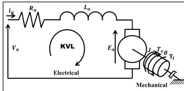
Fig. 10 DC motor schematic diagram
