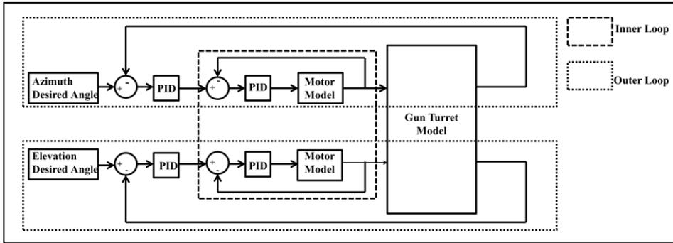
Fig. 9 Control structure for gun turret system
