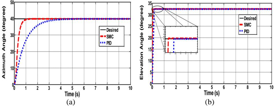
Fig. 14 Rotational angle of gun turret
