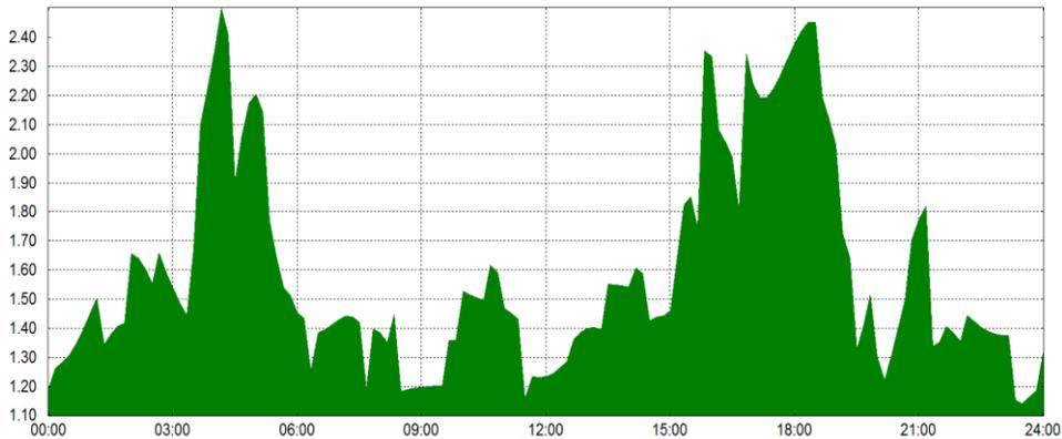
*Fig. 2 PDOP of GPS coverage at the test area for the period of the tests. The x-axis is UTC time while the y-axis is PDOP
