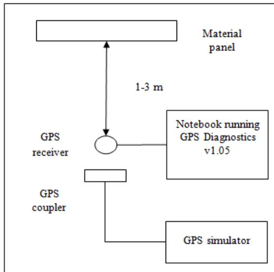
*Fig. 1 The test setup employed*
